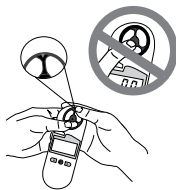
Replacing the Impeller
